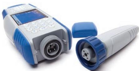
*RFID reader and handgrip can be connected to either side*
