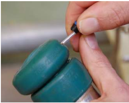
needle pierces 'straw' in liner
