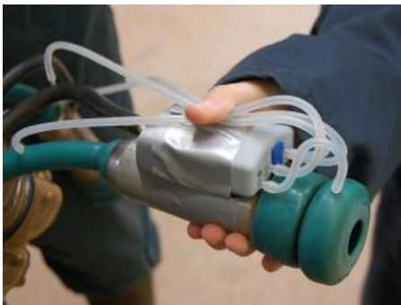
silicon tubes connect straws to VaDia
