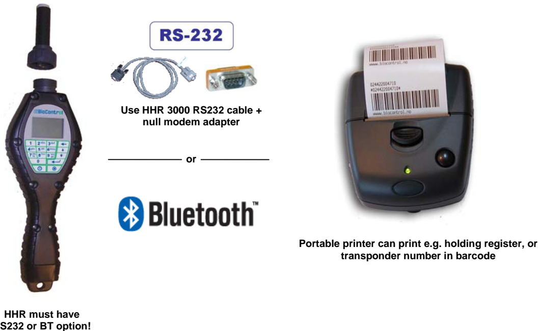
Figure 1: HHR-printer connection. Both RS232 and Bluetooth are available
