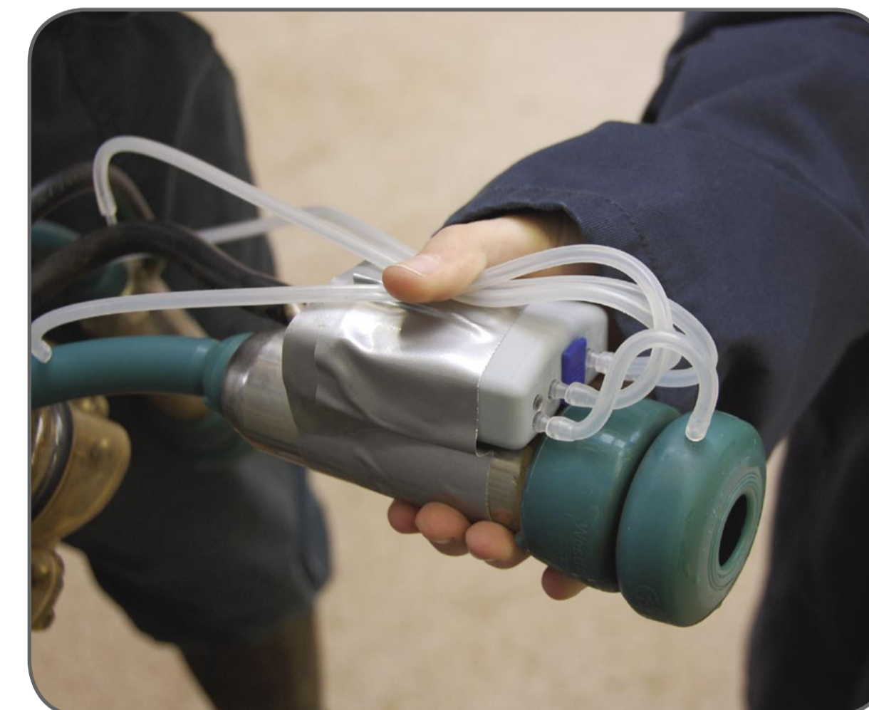
VaDia logger can be used on any type and brand of milking equipment, including robot
