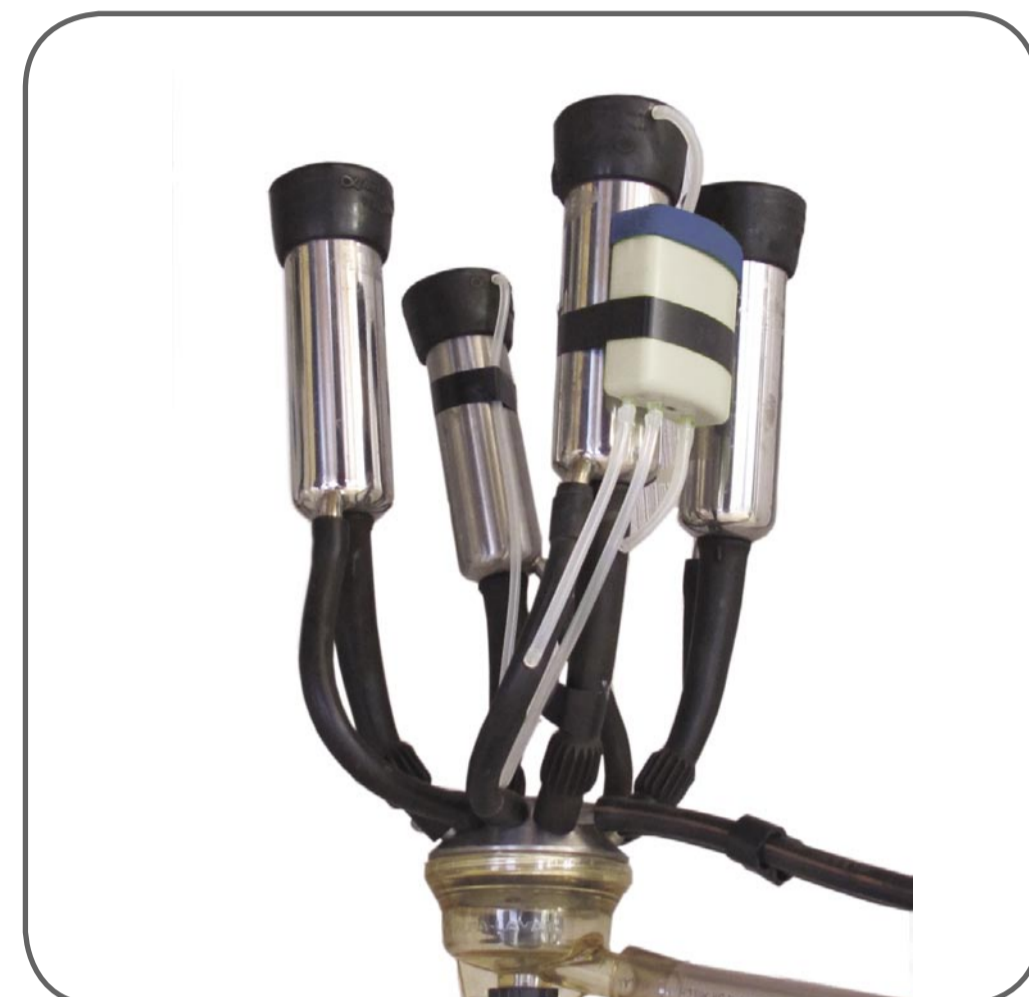
VaDia logs the vacuum at 4 points in the milking cluster
